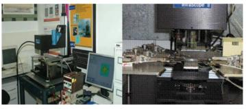
Quantum Focus microscope and micro-probe station
