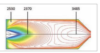
Combustion chamber temperature contours illustrating the flame shape. Image courtesy of Monitor Coatings Ltd and Southampton University
