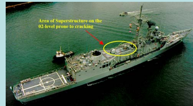
RAN Adelaide Class Frigate Repair of the main deck
